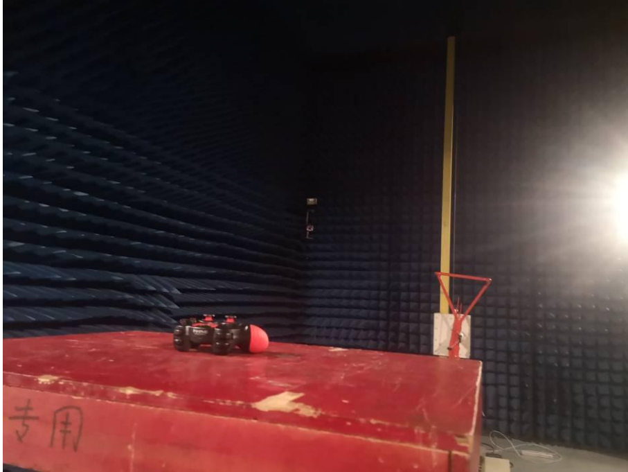
Radiated Emission Test Setup
